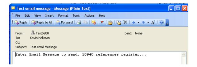
After communications the SMTP Send Register displays the email message number sent along with the results in the SMTP Status Register, 12318. 12318 changed to 0 after the initial write of a 1 to 12317, ending with a 1 after successful transmission:
