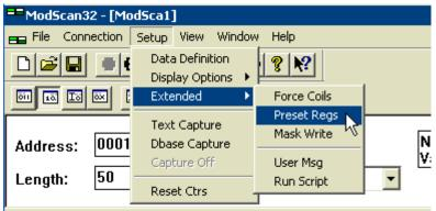
Figure 7.6: Write Multiple register (Preset Regs) selection
