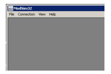
In order to activate the Modbus slave, you must select the Connection menu item and the method of the connection, Modbus/TCP Svr for network or the appropriate Port # for a serial port.
