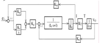
Figure1. Motor and current loop block diagram
