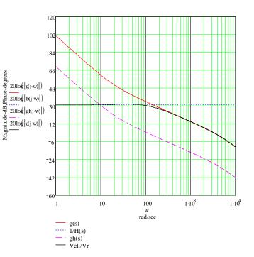
Figure 12. Velocity servo response
