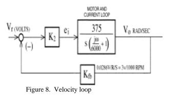
The servo compensation and amplifier gain are part of the block identified as  $K_2$ . Most industrial servo drives use proportional plus integral (PI) compensation. The amplifier and PI compensation can be represented as in figure 9[1].
