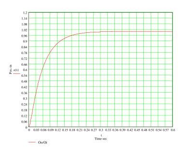
Figure 19. Transient response with Acceleration feedback
