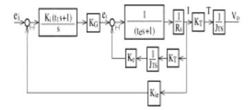
Figure 2. Equivalent motor and current loop Block diagram
