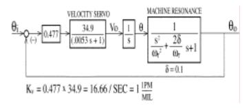
Figure13. Position loop block diagram
