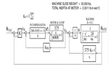
Figure 17. Equivalent Industrial BLDC servo drive with a 10 Hz resonance in the machine structure and acceleration feedback
