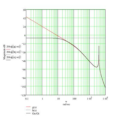
Figure 18. Position frequency response with acceleration feedback
