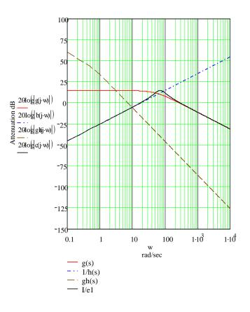
Figure 3. Current inner loop
