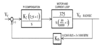
Figure 11. Velocity loop with PI compensation
