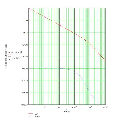
Figure 7. Motor and I loop frequency Response
